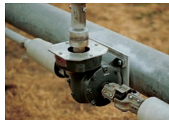
Center drive powered by the spinner mechanism.
